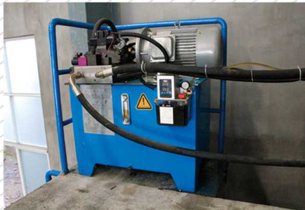
油箱总成——油泵;电磁阀等均采用台湾进口原件 Oil Tank Assembly:including Oil Pump,Electromagnetic Valve and other ompnents adopted rae imported from Taiwan.
