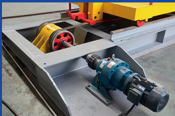
③ 台车变频调速 frequency speed control of worktable
