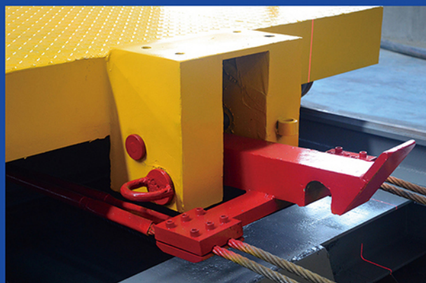
④ 台车牵引装置 Coupling device of worktable
