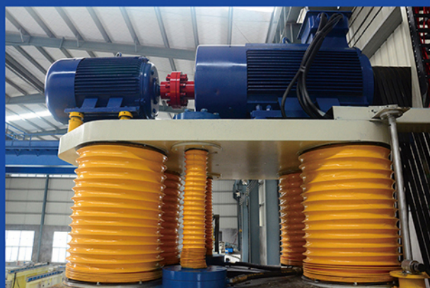
② 双电机驱动装置 Moved by dual motors
